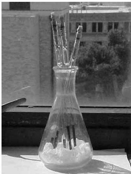
FIG. 2. Medium pressure NMR sample tubes containing solutions of the diiron complexes, pressurized with 10 bar D_2 and were exposed to sunlight on the windowsill.
